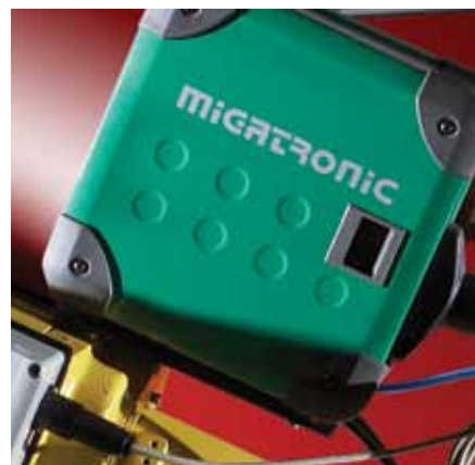
RWF - Robot Wire Feeder.
